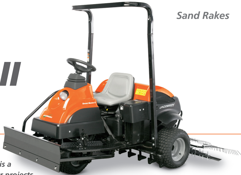
Groom Master® II gas shown with front blade, cultivator and rear rake
